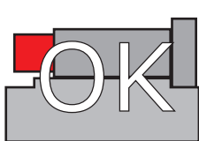
Ferrule CORRECTLY Located
